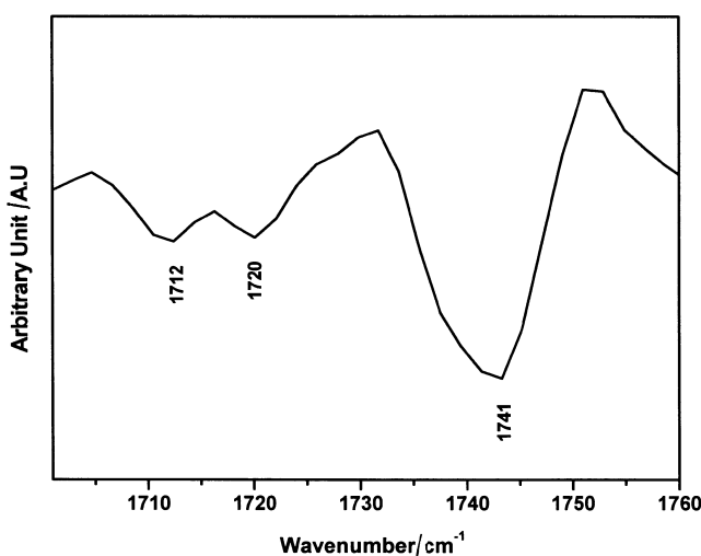
Figure 3. The second derivative spectra of MHOCPOOB in the 1760–1700 \text{cm}^{-1} region.
